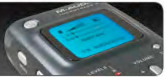
**Power Button:** Press and hold this button for approximately one second to turn MicroTrack II on and off. *Should the unit ever become unresponsive, pressing and holding this button for approximately ten seconds forces MicroTrack II to shutdown.*
