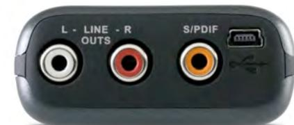
USB Input: Connect MicroTrack II to a host computer or to the included USB power supply using this input.
